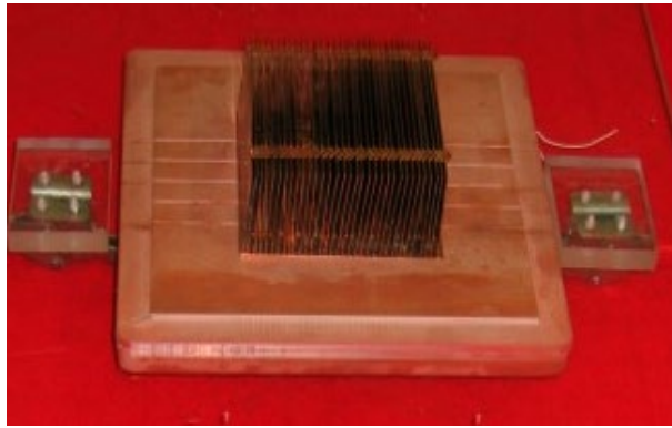
Figure 5. Photograph and drawing of high performance fine-pitch copper base-copper fin air-cooled heat sink. W=82 mm; L=90 mm; H=43 mm; b=1.5 mm; t=0.4 mm.
